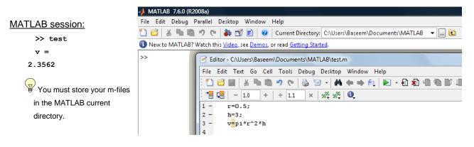
Example 2: Write a function to calculate the volume of a cylinder given its radius and height. Test your function with r=0.5 m and h=3 m.
