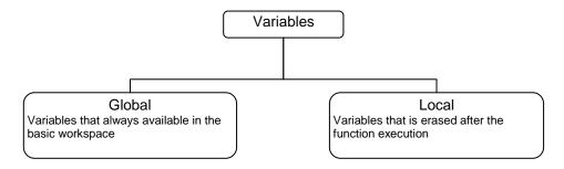
Use the <u>global</u> command to share variables between the command window or script files and function files. The global command should be inserted at the beginning of each one to determine which variables are shared.
